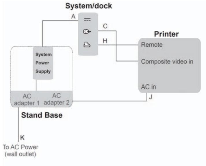
Figure 1 Connectivity of printer and system
