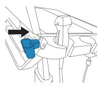
2. Slot the microphone into the mounting fixture.
