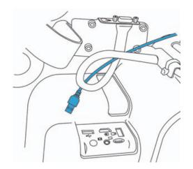
Insert the USB cable into a USB port on the back of the system.
